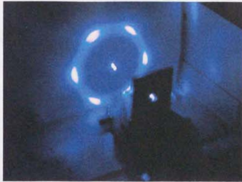
Figure 3.10: Laser diffraction pattern of ordered polystyrene particles. The structure is close-packed hexagonally.
